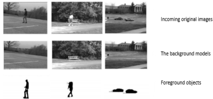
Figure 3.9: An example of background subtraction and extraction silhouettes of foreground objects moving in three different images.
