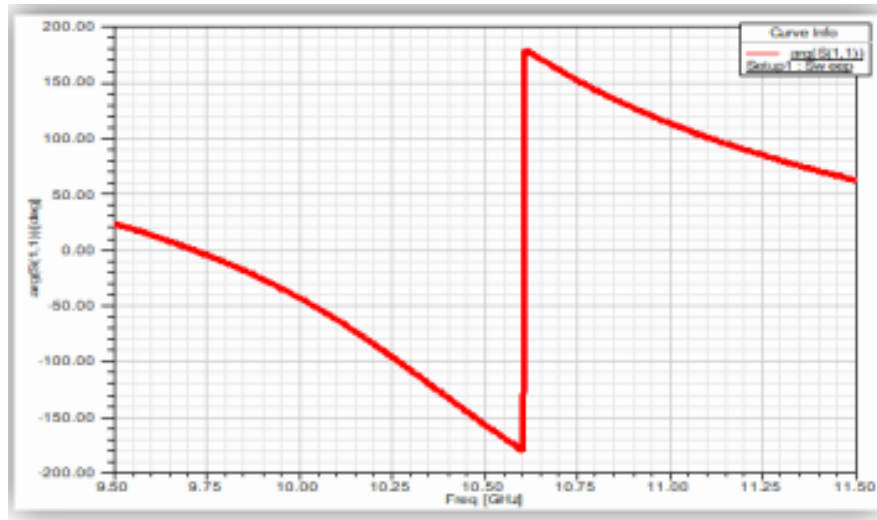
Figure 2.15: Phase response of the volume resonator for dimensioning the quality factor.
