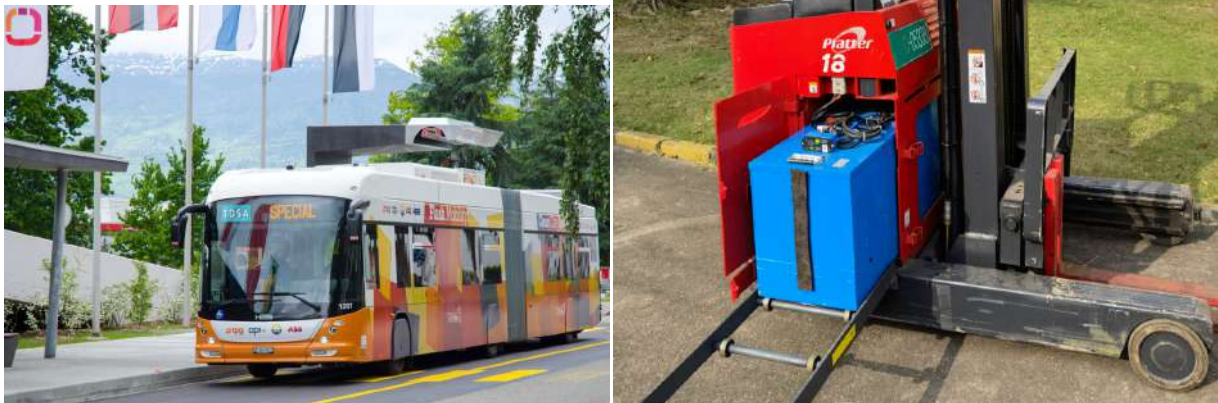
(a) Flash chargers using supercapacitors are provided at ABB TOSA bus stops.
