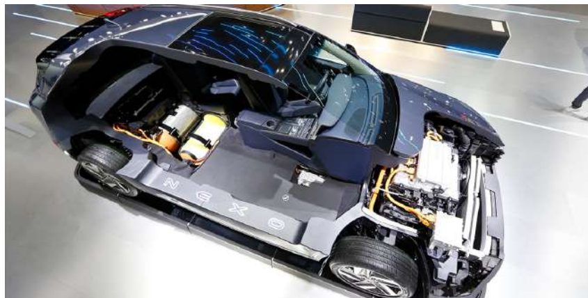
(b) A cutaway model of the Hyundai Nexo fuel cell electric vehicle
