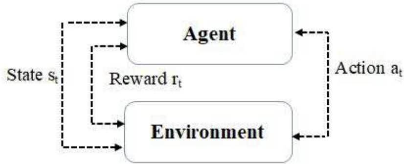
Figure 1.16: In the reinforcement learning framework, an agent performs a sequence of actions, with each action resulting in both a reward and a new state
