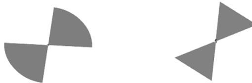
Figure I.17 Antenne papillon
