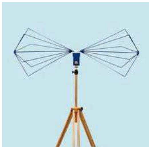
Figure 5.8 Antennes bi-coniques [22]
